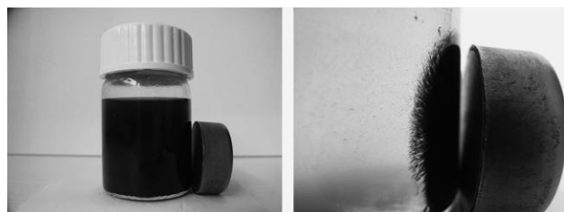
Figure 4. Magnetic separation of finely dispersed superparamagnetic catalytically active nanoparticles (left: shortly after the application of the magnet; right: 2 min later).
